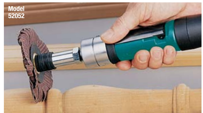
52052 Lightweight Dyninger with single arbor-mount star attached.
