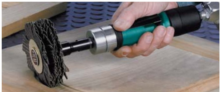
Lightweight Dyninger with Spindle-Mount Sanding Stars.
