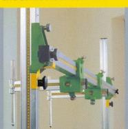
McPherson strut bridge is made entirely of steel because this is the only material able to guarantee precise measurement of the shock absorbers. It is easily mounted on the crossbeam and, naturally, all dimensions are indicated on the data sheet. Moreover, it is possible to control the external panels and hinges. Thanks to the yellow support hooks, one person is all it takes to install the bridge.
