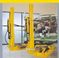
The articulated pulling tower (optional), paired with the fixed tower, is useful when you need to perform two simultaneous pulls close together. The internal tower mechanism is made up of seven bearings to ensure perfect sliding.
