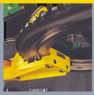
The mounting mechanism on the pulling tower has been patented because it ensures easy sliding, not only along the sides but, above all, around curves where it is always perpendicular to the bench.
