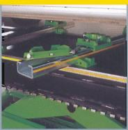
These flanges make it possible to remove any crossbeam re-position during the course of repairs.
