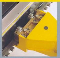
The advanced technology used to build the pulling towers ensures perfect sliding, even after years of work. The pulling towers do not ever have to be removed or dismounted. They slide freely all around the bench and can be blocked at 60 mm intervals. The pulling power remains constant at all heights, the chain always working in a horizontal position.
