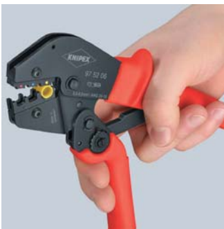
First step: move the handle with two fingers only until both jaws touch the connector to be crimped
