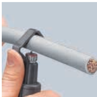
Setting the tool for circular cut
