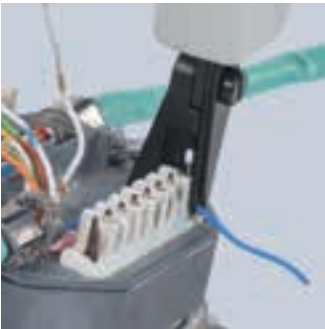
Inserts and cuts cables in one operation
