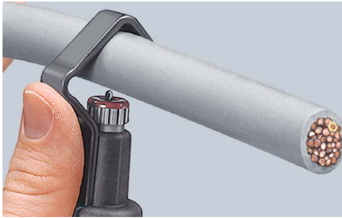
Setting the tool for circular cutting
