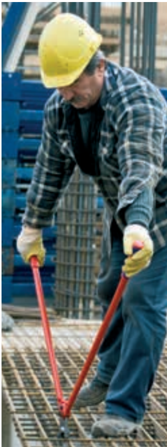
The special shape of the mesh cutter head, 71 82 950, enables it to cut structural steel that is lying down flat
