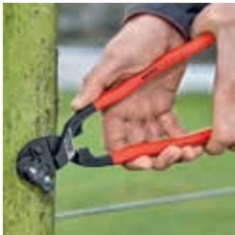
Two-hand operation for maximum cutting force
