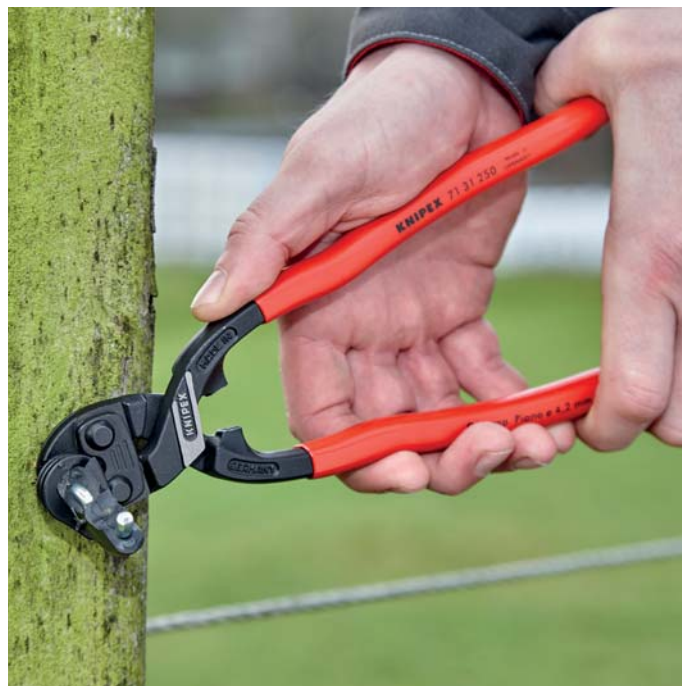
Two-hand operation for maximum cutting force
