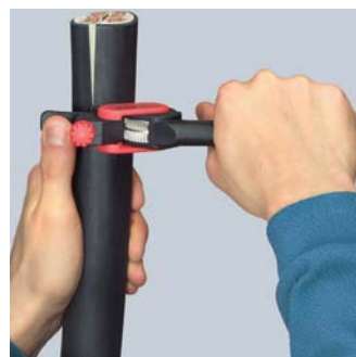
Turning the tool for circumferential cut
