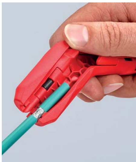
Dismantling of a data cable
