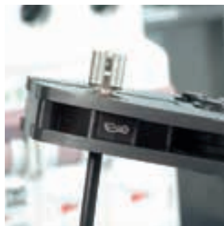
Clearly visible marking on the crimping dies with pictograms
