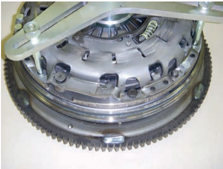
13. Tension disc springs.
