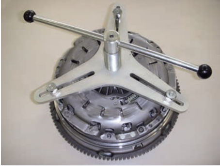
10. Guide the SAC clamping device over the threaded bolts.
