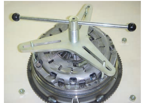
15. Loosen hexagonal nuts - remove clamping device.
