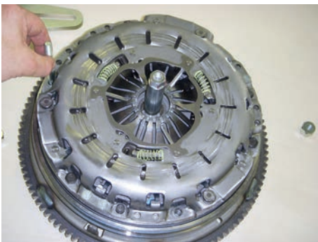
16. Remove threaded bolts.
