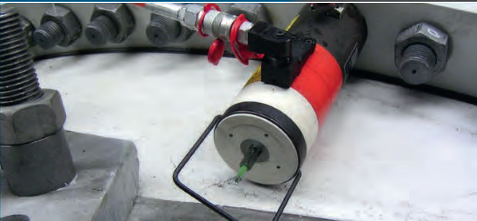
Single stage design for situations whereby the area around the axis is cramped
