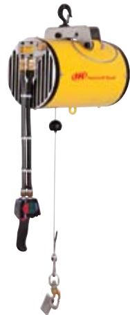
Z Stop: The optional Z Stop is a patented device that will eliminate the down-drift of suspended loads or tools during shut down or at night when the air supply is shut off. The Z Stop will stop drift within 6 inches (152.4 mm) and put the Balance Air into a mechanically locked position preventing damage to tools or objects below the suspended load. Available for use on all 10 inch (254 mm) diameter units.
