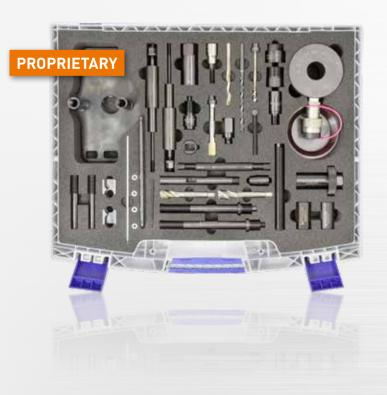
**Use:** For removing frozen common rail injectors from the cylinder head using a 20 ton hollow piston cylinder. If the injector tears during the extraction at the bottom screw connection, is it possible to pull the rest of the injector using the additional extraction spindles.
