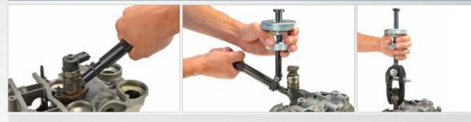
For non-destructive removal of various slightly and moderately jammed injectors.
