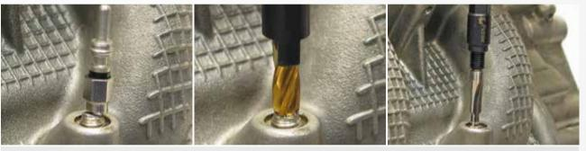
Tools for removing glow plugs and for cleaning or reworking the glow plug hole.
